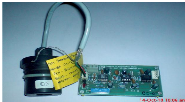
Fig. 3 Photograph of CO-CF Sensor Module.
